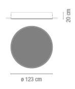
Electrical characteristics 2 x G5 230V 24W (T5) AND 2 x G5 230V 39W (T5) AND 2 x G5 230V 54W (T5)
