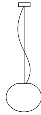
S5 Ceiling Rose Ø 120 mm Ceiling rose LED Ø 160 mm Ceiling rose LED DIMM Ø 200 mm Cable 2000 mm Diffuser Ø 360 mm H 285 mm
