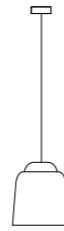
S5 Ceiling Rose Ø 120 mm Cable 3000 mm Diffuser Ø 360 mm H 400 mm
