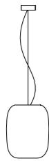
S5 Ceiling Rose Ø 120 mm Ceiling Rose LED Ø 160 mm Cable 2000 mm Diffuser Ø 360 mm H 450 mm
