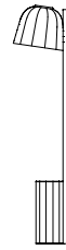
T1 USB H 600 mm Diffuser Ø 130 mm H 110 mm Base Ø 80 mm
