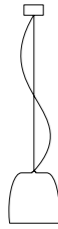
S1 Ceiling Rose Ø 80 mm Ceiling Rose LED Ø 160 mm H 45 mm Ceiling Rose LED DIMM Ø 200 mm H 45 mm Cable 2000 mm Diffuser Ø 210 mm H 210 mm
