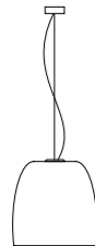
S7 Ceiling Rose Ø 120 mm Ceiling Rose LED Ø 160 mm Ceiling Rose LED DIMM Ø 200 mm Cable 3000 mm Diffuser Ø 480 mm H 490 mm
