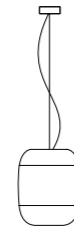
S5 Ceiling Rose Ø 120 mm Ceiling Rose LED Ø 160 mm Ceiling Rose LED DIMM Ø 200 mm Cable 2000 mm Diffuser Ø 360 mm H 450 mm
