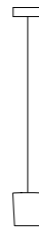
S1 Ceiling Rose Ø 120 mm H 40 mm Cable 3000 mm Diffuser Ø 135 mm H 150 mm
