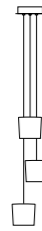
3R - 3S Ceiling Rose Ø 180 mm H 40 mm Cable 3000 mm Diffuser Ø 135 mm H 150 mm
