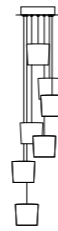
7R - 7S Ceiling Rose Ø 240 mm H 40 mm Cable 3000 mm Diffuser Ø 135 mm H 150 mm
