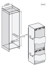
KFN7795D, built-in (footnote\*) (installation drawings)
