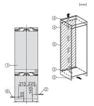
KFN7795D, installation (footnote\*) (installation drawings)
