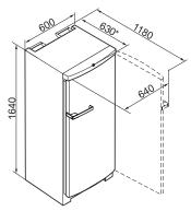
FN12621S-1, FN26062, FN26065 (installation drawings) (\*footnote)
