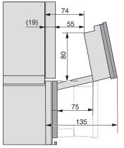
DGC7x4x, DGC7x4x-55, DGC7xxx, DGC7x4xHCPro, DGC7x4xHCXPro installation drawings
