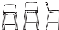
Stackable stool with high back L 51 P 54 H 94-104 cm W 20 1/8 " D 21 2/8 " H 37-41"
