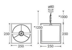
Dimensions in mm and approximate \*Adjustable flex and chain length
