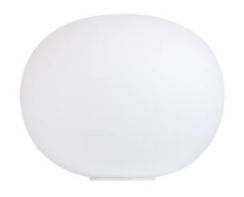
Table/desk lamp providing diffused light. Diffuser consisting of an externally acidetched, hand blown, flashed opaline glass and a die-cast aluminum threaded ring nut with alodine plating finish. 30% fiberglass reinforced injection-molded polyamide base. Gray painted, die-cast aluminum diffuser support. On the cable there is the electronic dimmer which allows the regulation of light brightness.
