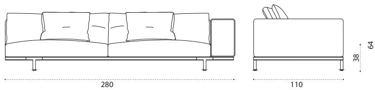
→ 65 | 1 box 282X112X67H 85 Kg | NOTE: this product can also be shipped disassembled
