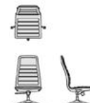
LS_45 cm. 66x66x45,5/103,5min - 54,5/112,5max h inch 26 1 / 2 x26 1 / 2 x18 3 / 4 /40 3 / 4 min - 21 1 / 2 /44 1 / 4 max h
